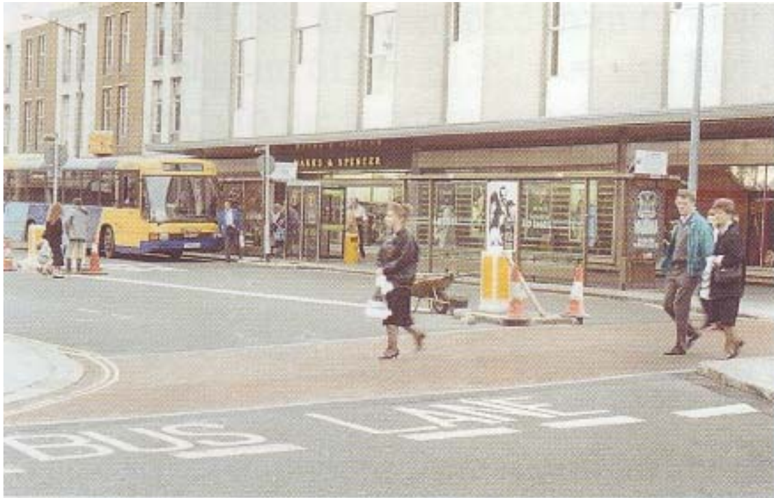
Different colour or texture of road surface can encourage compliance and ease enforcement
